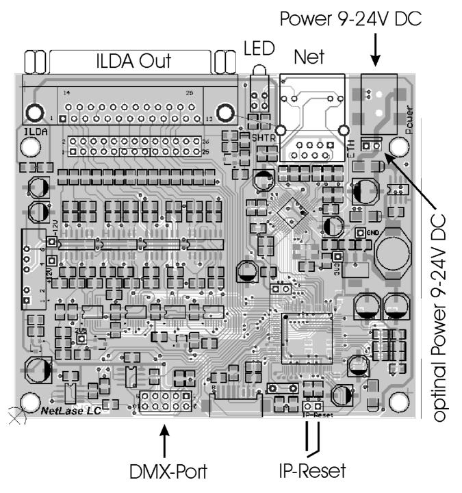
Power can be connected at the front connector or at the additional 2pin connector. Power input is reverse voltage protected.
