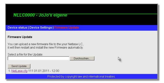
Do NOT change any settings or do a firmwareupdate, while an output session is running! This can cause malfunction of the application and/or NetLase LC card.
