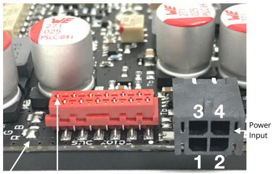
Jumper 1/2 Pin 1 Modulation Input
