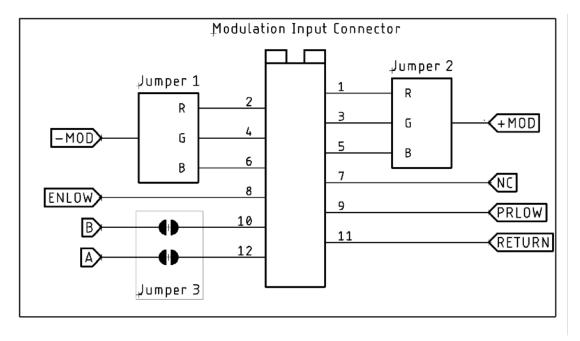
**Jumpers:** Please consider that the jumpers are preconfigured to match the wavelenght e.g. a 638nm red lasermodule will always use pin 1 and 2 for modulation, a green 520nm module will always ship with jumpers preconfigured to use pin 3/4 as modulation inputs.
