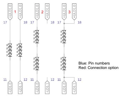
Option 1 uses both channels to drive eight diodes. Because of the four diodes per string arrangement, the driver only needs (5V\*4)+3V= 23V VCC min. The disadvantages are increased overall current, resulting in less efficient operation.
