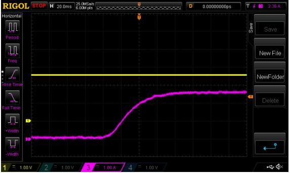
Turn on event e.g. connecting 48V to tuned driver with modulation signal already in place with 2.5V modulation signal and Imax tuned to 5A. No overshoot and 65ms softstart time
